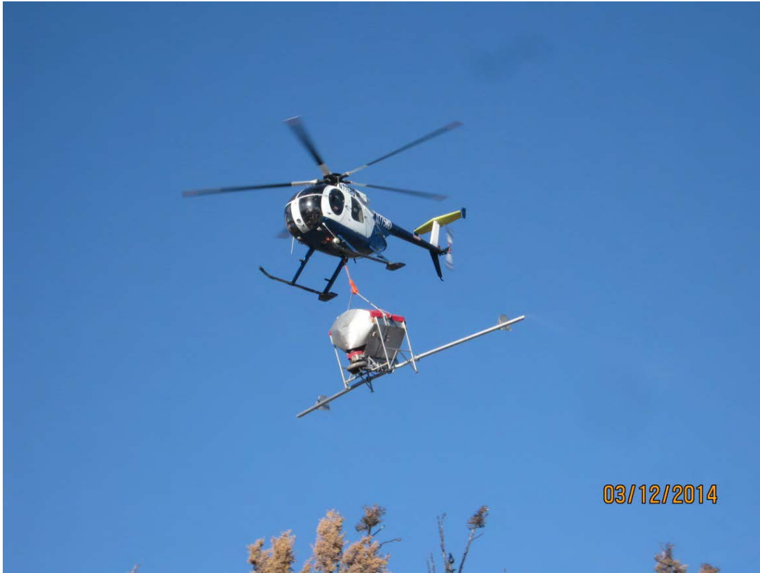
The photo at left is of the contract helicopter applying sagebrush seed on the State Fire.
